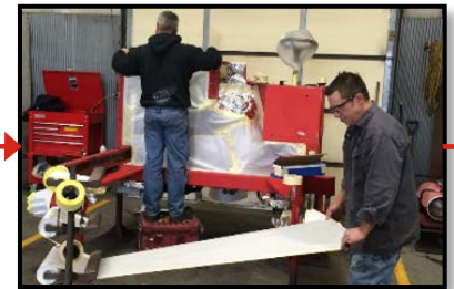
Wash, Sand, & Prep for Paint
